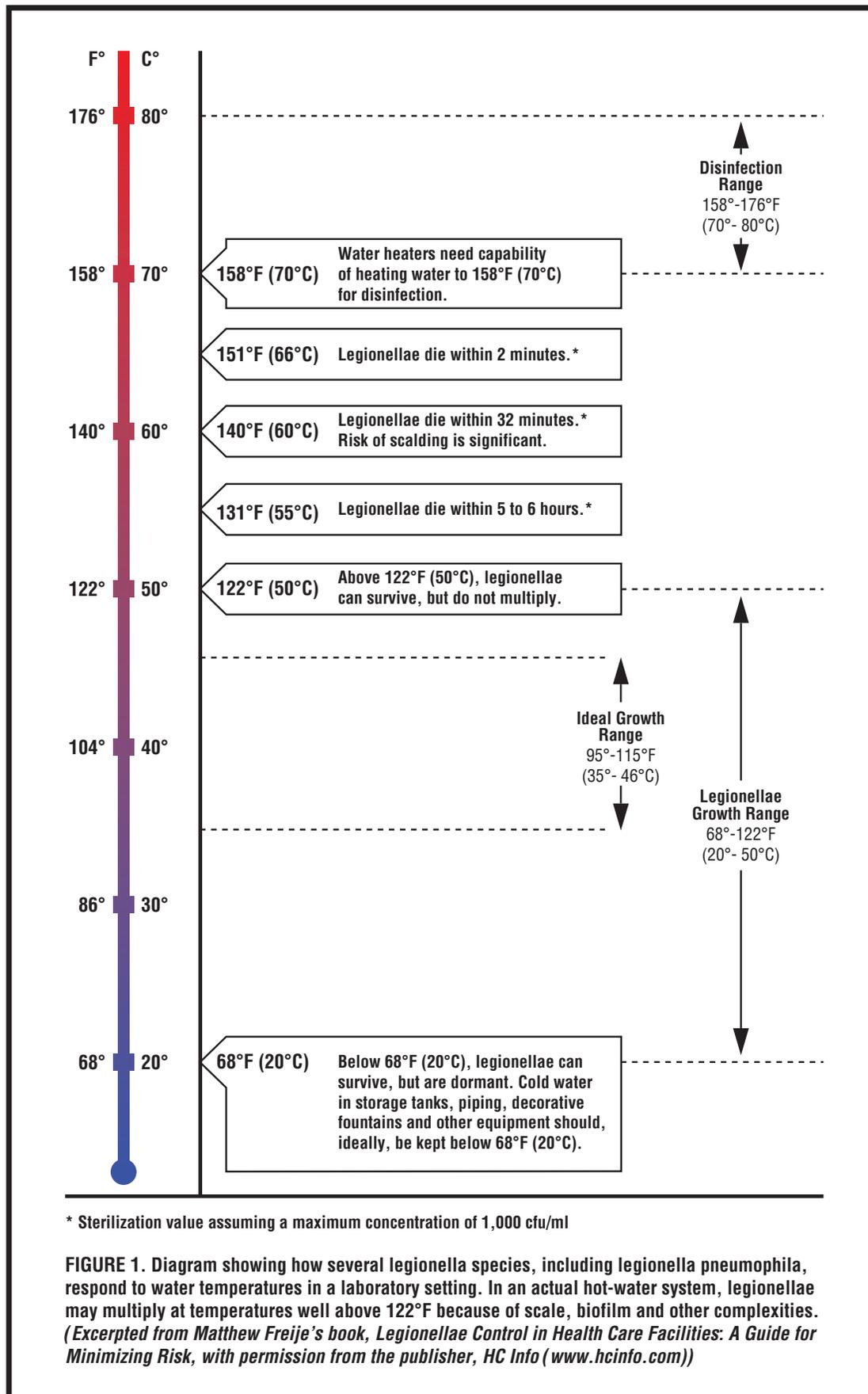
Figure 2 – Water Temperature vs Scald Potential
