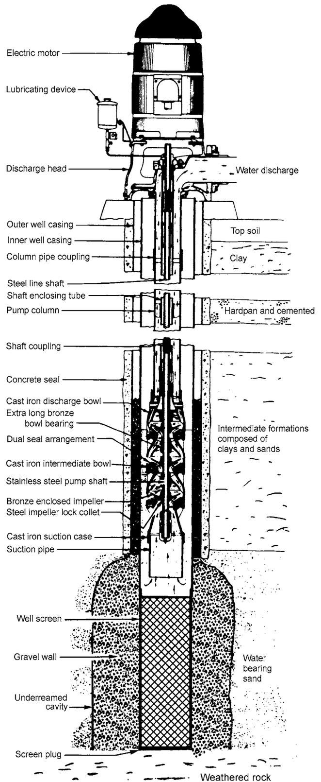
**Figure 9-4 Typical Gravel Filter Well with a Vertical Turbine Pump**
