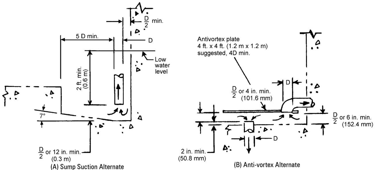
Figure 9-5 Storage Tank Suction Piping Detail
