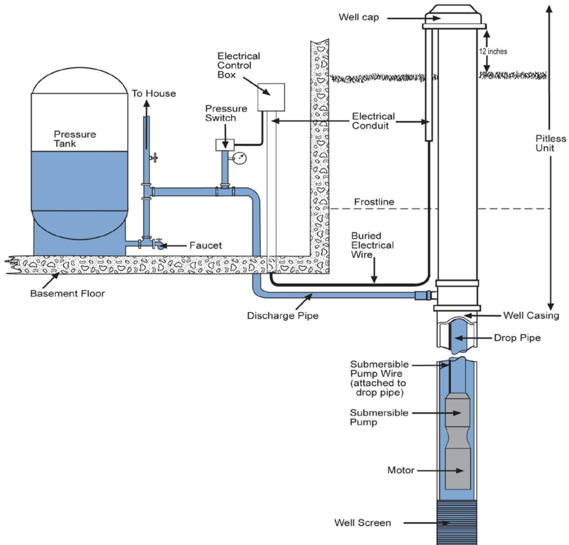
**Figure 9-3 Well and Water System**
