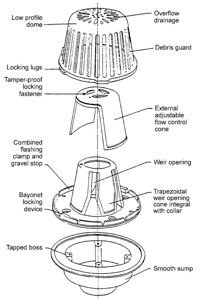
**Figure 4-9 Example of a Controlled-flow Drain**
