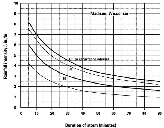
Figure 4-3 Intensity-Duration-Frequency Curve
