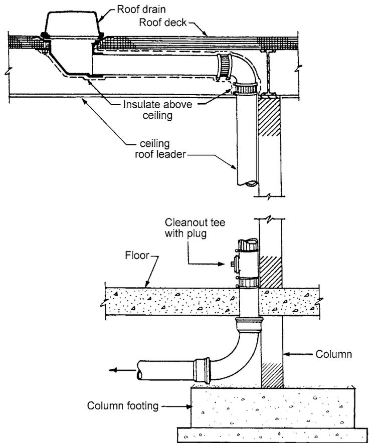
**Figure 4-8 Typical Roof Drain and Roof Leader**
