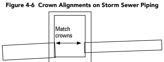
**Figure 4-6 Crown Alignments on Storm Sewer Piping**
