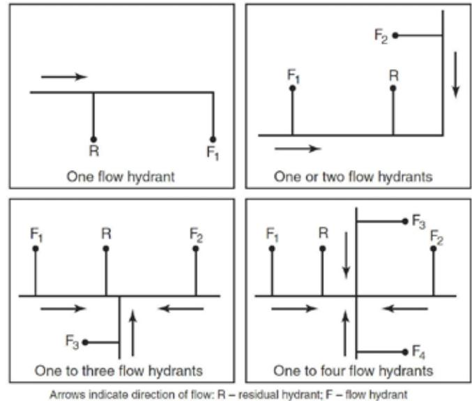
Figure 1-3 Method of Conducting Flow Tests
