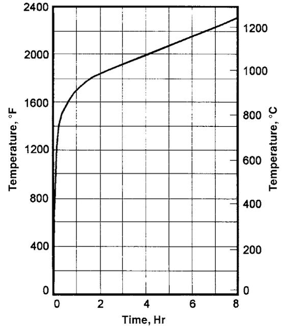
Figure 1-1 Time/Temperature Curve for Standard Fire Test
