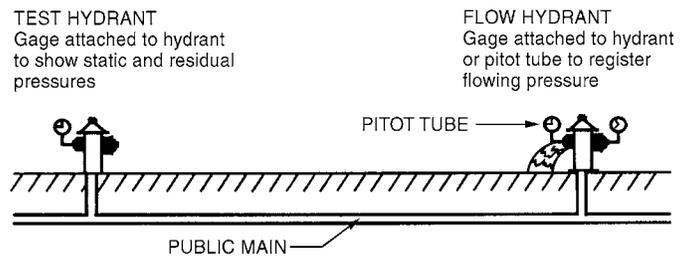
Figure 1-2 Pitot Tube Position
