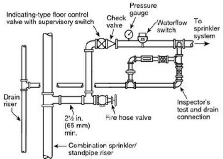
Figure 1-17 Acceptable Piping Arrangement for Combined Sprinkler/Standpipe Systems
