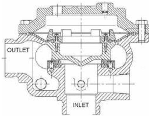
Figure 1-12 Deluge Valve with a Single Differential Diaphragm
