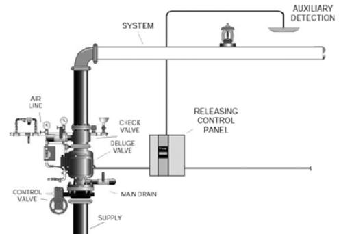
Figure 1-10 Preaction Valve Riser
