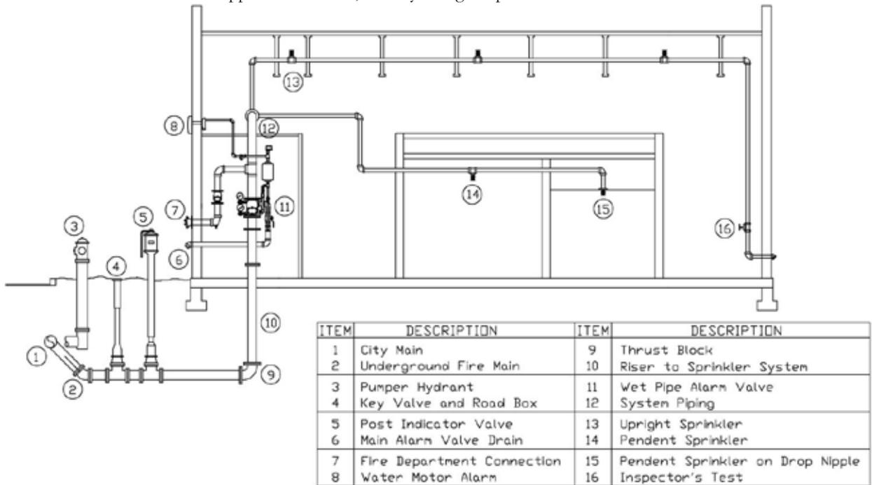
Figure 1-6 Wet Pipe Sprinkler System
