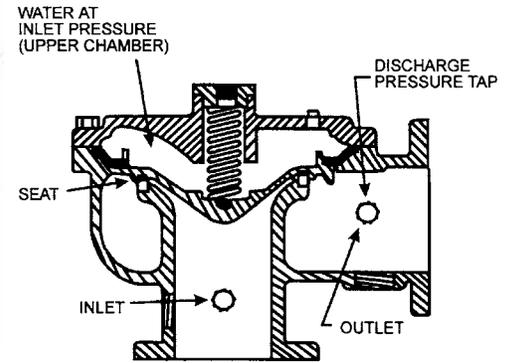
Figure 1-13 Deluge Valve with Outlet Pressure Regulator
