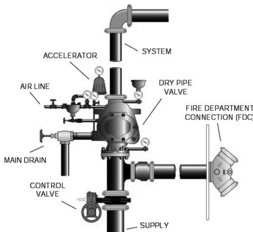
**Figure 1-9 Dry Pipe Valve Riser**
