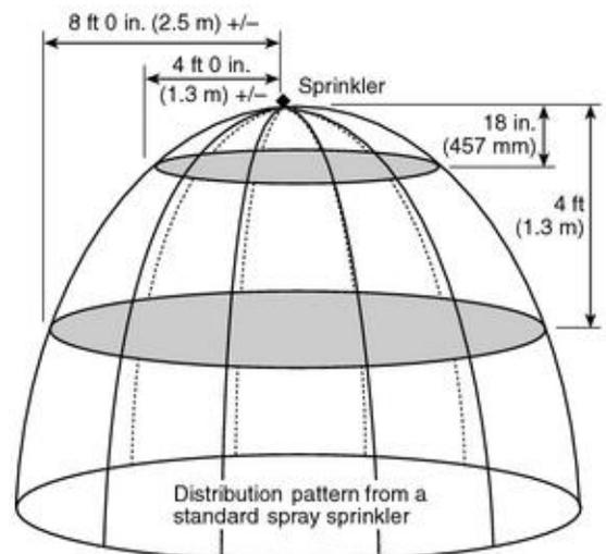
Figure 1-16 Example Sprinkler Flow Pattern
