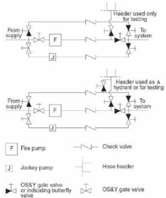
Figure 1-19 Fire Pump System
