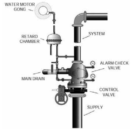
Figure 1-5 Typical Alarm Check Valve Riser
