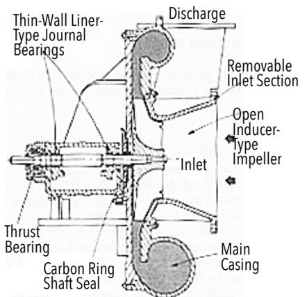
Figure 14-8 Centrifugal Compressor
