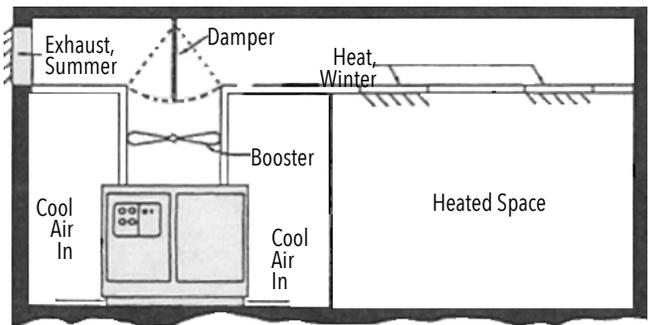
**Figure 14-19 Using Air-Cooled Screw Compressor Heat**
