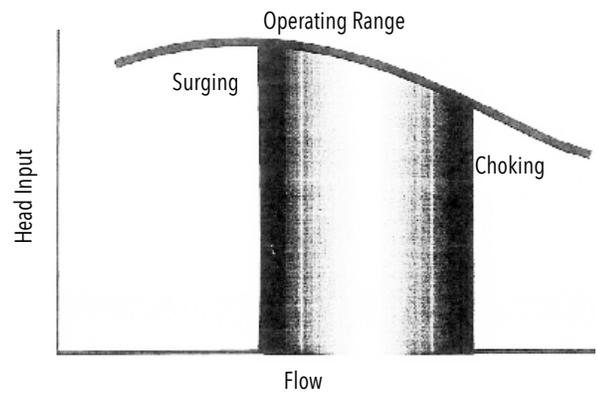
Figure 14-16 Centrifugal Curve
