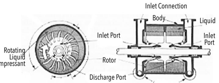
Figure 14-5 Liquid-Sealed Rotary Compressor, Circular Lobe
