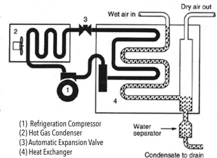
Figure 14-12 Refrigerated Air Dryer
