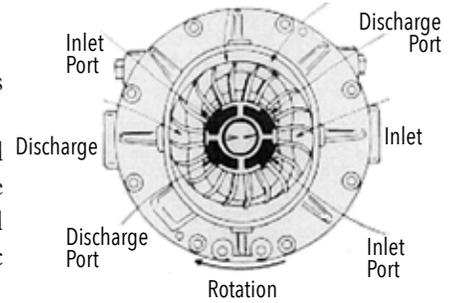
Figure 14-6 Liquid-Sealed Rotary Compressor, Double Lobe
