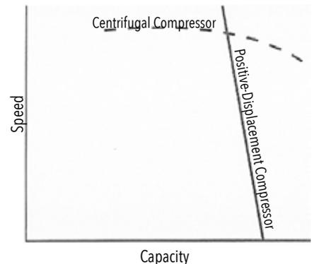
**Figure 14-15 Centrifugal vs. Positive-Displacement Compressor Curves**
