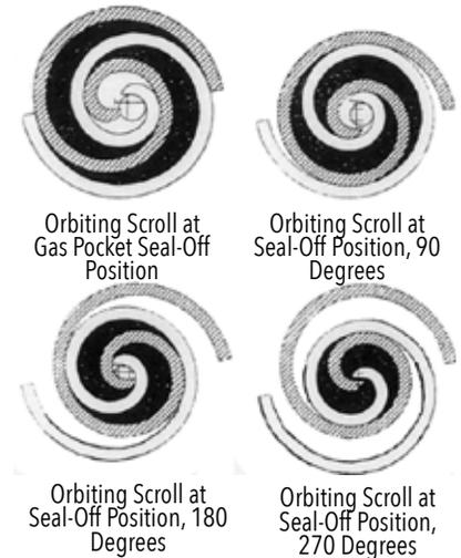
Figure 14-7 Operating Positions of Scroll Compressors
