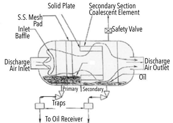
Figure 14-9 Coalescing-Type Oil Separator
