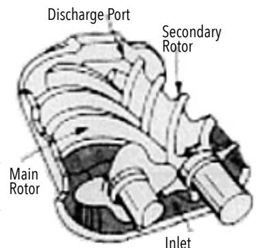
**Figure 14-4 Rotary Screw Compressor**
