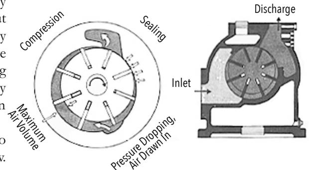
**Figure 14-3 Sliding Vane Compressor**
