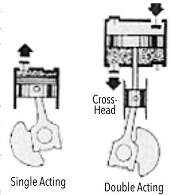
**Figure 14-2 Single- and Double-Acting Cylinders**
