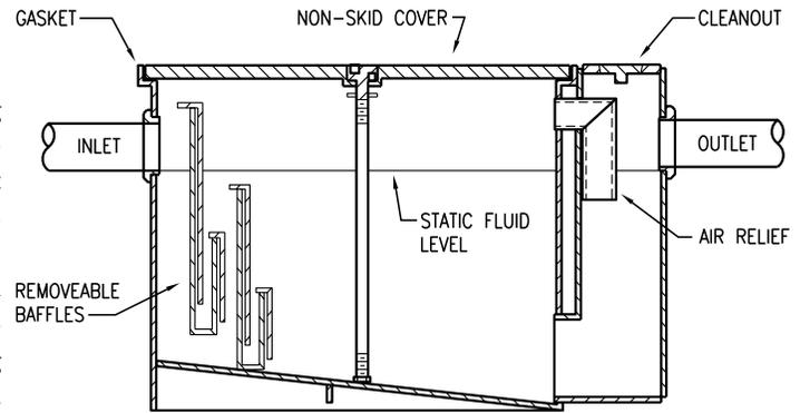
Figure 8-4 Hydromechanical Grease Interceptor
