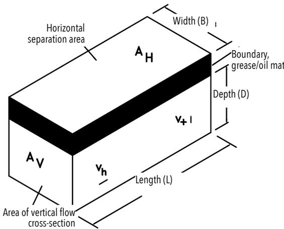
**Figure 8-2 Cross-Section of a Grease Interceptor Chamber**
