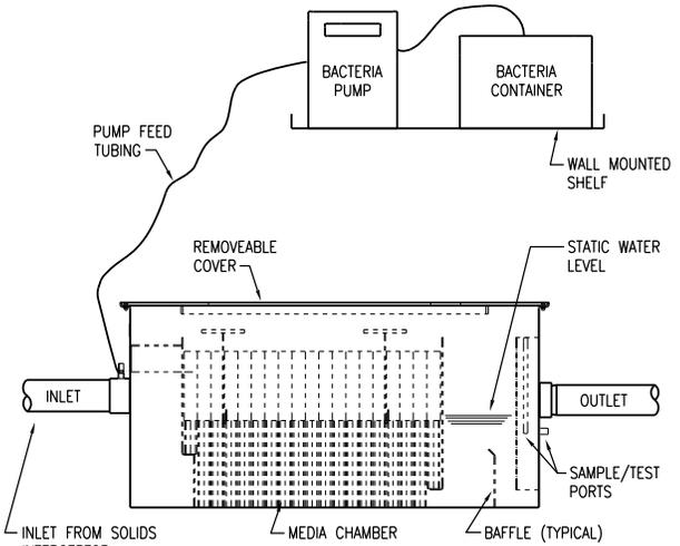
Figure 8-6 Bioremediation FOG Disposal System
