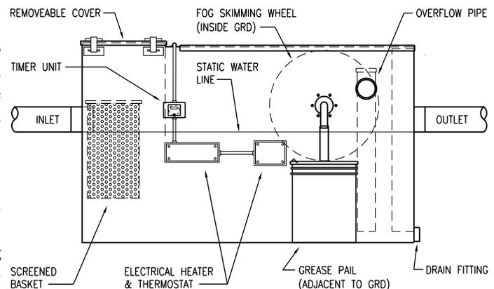
Figure 8-5 Timer-Controlled Grease Removal Device
