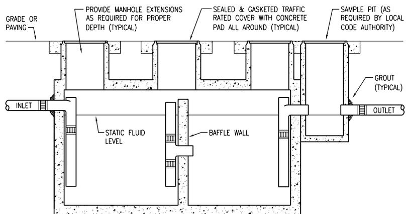
Figure 8-7 Gravity Grease Interceptor
