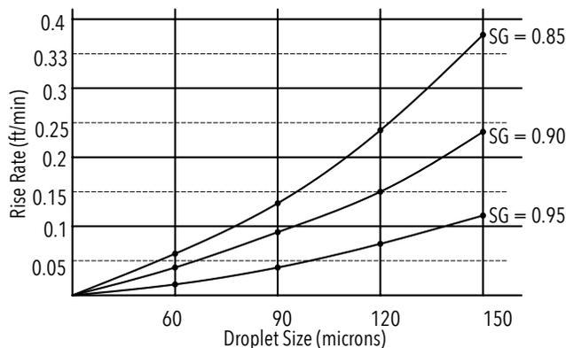
Figure 8-1 Rising and Settling Rates in Still Water
