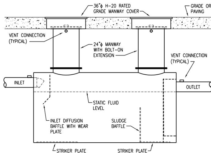
**Figure 8-8 Prefabricated Steel Gravity Grease Interceptor**
