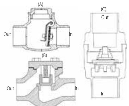
**Figure 3-8 Check Valves: (A) Swing, (B) Lift, and (C) Spring Loaded**
