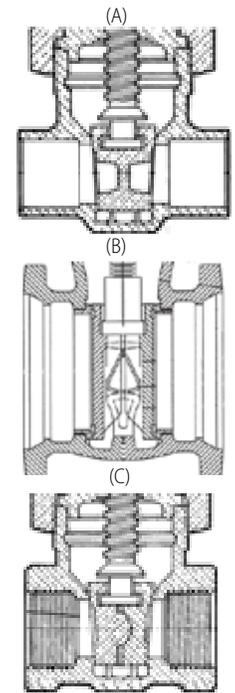
**Figure 3-2 Gate Valve Discs: (A) Solid, (B) Double, and (C) Split Wedge**
